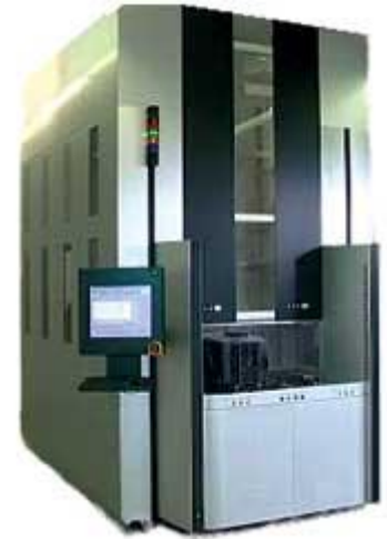
Figure 1. This stocker, sorter and cassette buffer for 300-mm wafers exemplifies advances in single-wafer management. Wafers are insulated from the environment and continuously purged with filtered air or nitrogen. Source: Tec-Sem.
